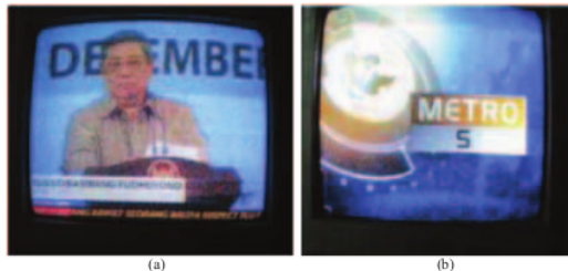
Fig.10: The quality of TV trainer reception using an L-dipole antenna
